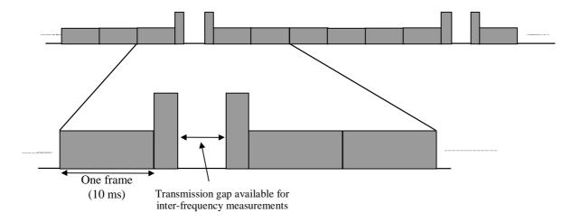
Figure 11: Compressed mode transmission
